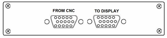
Connect your LCD monitor VGA cable (not supplied) to the plug labeled "**TO DISPLAY**"
