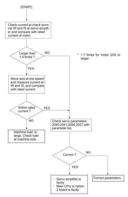
From 1st axis to 4th axis are main CPU board. 5th axis or later are option 2 board.
