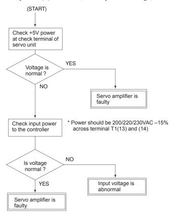
2) Servo amp LED [3] turns on (DC power shortage)
