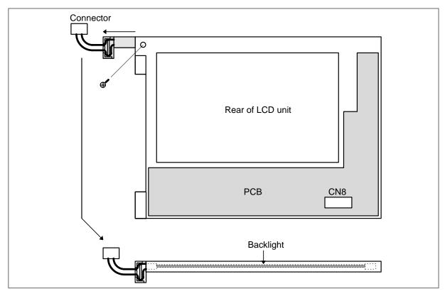
3)–3 For the 7.2" and 9.5" LCD units (monochrome) manufactured by Hitachi
