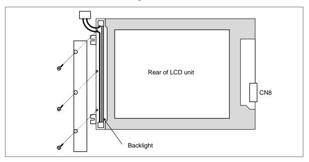
3)-2 For the 10.4" LCD unit (color) (old type)As shown below, remove the screw, and pull out the case containing the backlight. Replace the backlight with a new one.
