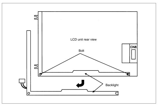
4) Upon completion of replacement, reassemble the unit by reversing the steps 1 through 3 above.
