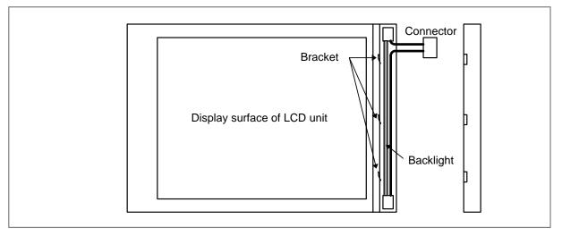
3)–4 For the 7.2" LCD unit (monochrome) manufactured by Sharp Remove the three screws from the left part on the front of the LCD unit, and remove the cover. Then, the backlight is exposed. Replace the backlight with a new one.
