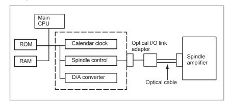
System control module is faulty. (Bold line in the figure below indicates module mounting position.)
