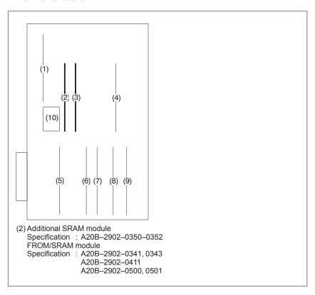
(3) Low voltage of memory back up battery. Battery alarm occurs if voltage is 2.6V or less (3.0V rating).
