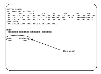
(a) If the address falls in a range of 0F1000H to 0F5FFFH, 740000H to 77FFFFH, or 7C0000H to 7FFFFFH:
