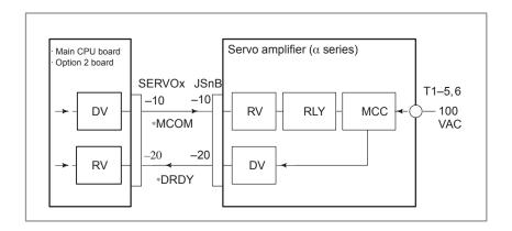
From 1st axis to 4th axis are main CPU board. 5th axis or later are option 2 board.
